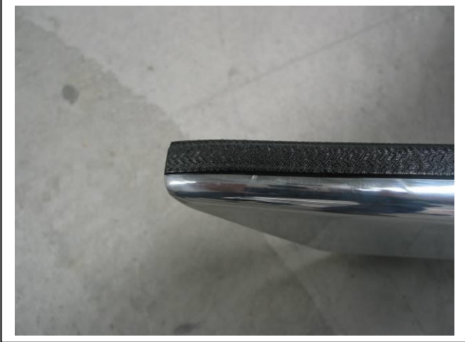
Figure 9: Cut end to match channel end
