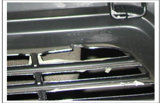
Figure 4: Cut out in plastic bumper. Rear of driver's side shown
