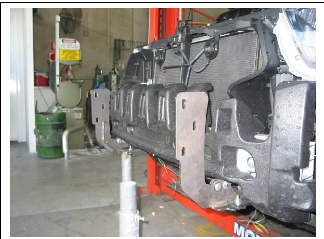
Figure 5: External mounts fitted with bar removed for photo
