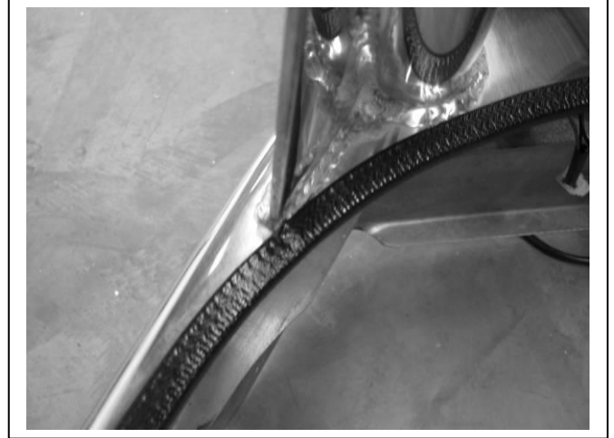
Figure 10: Clip lock beside tube gussets
